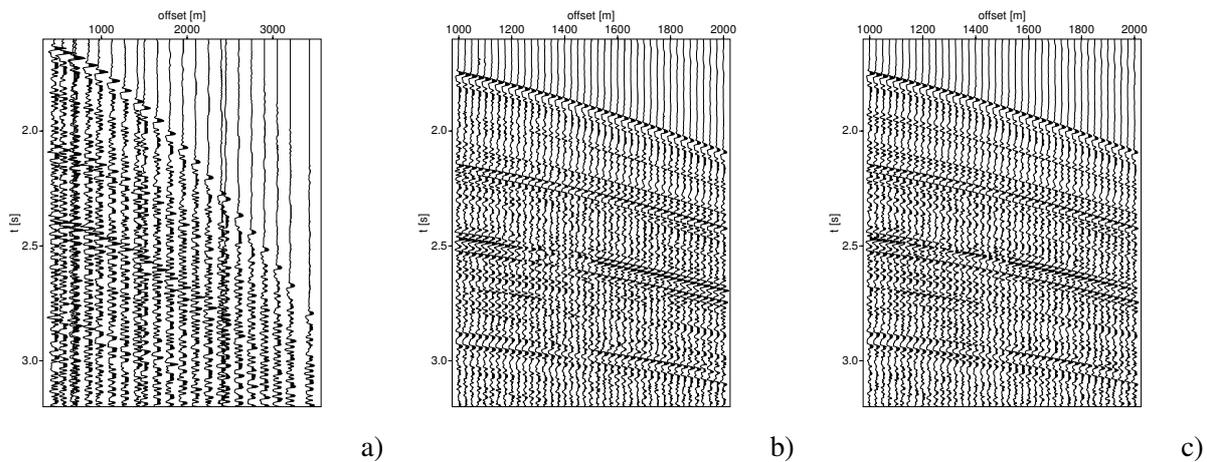
Figure 1: real data example: a) original CMP gather of the prestack data, b) interpolated CMP gather using a separate search of the parameters  $b_1$  and  $a_{11}$  in the first step, c) interpolated CMP gather using a simultaneous search of the parameters  $b_1$  and  $a_{11}$  in the first step.
