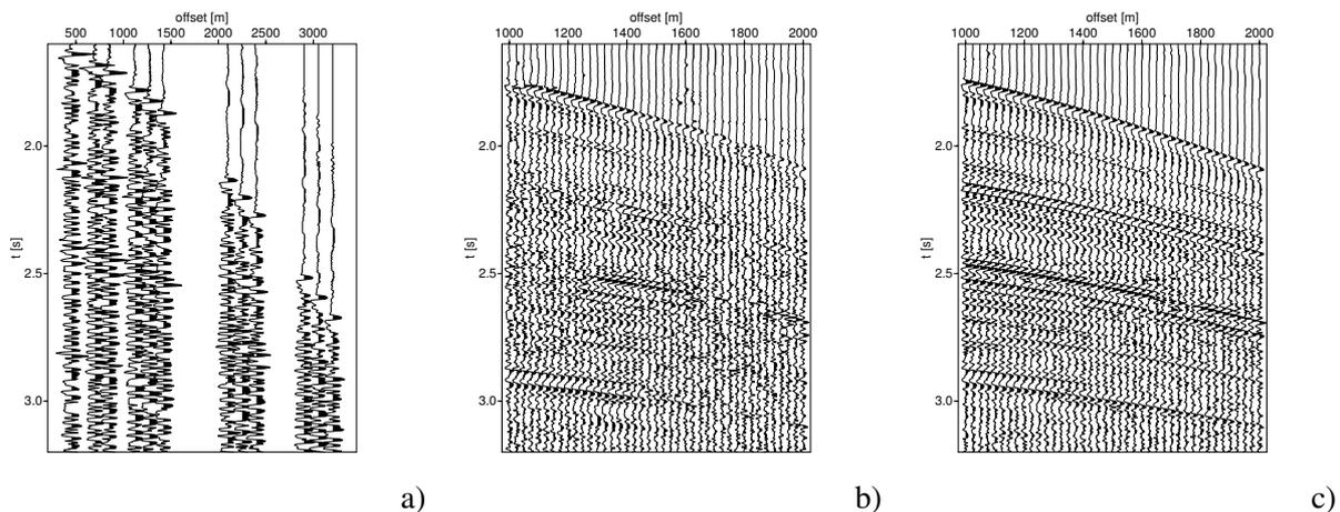
Figure 2: real data example with large gaps: a) original CMP gather of the prestack data, b) interpolated CMP gather using a separate search of the parameters  $b_1$  and  $a_{11}$  in the first step, c) interpolated CMP gather using a simultaneous search of the parameters  $b_1$  and  $a_{11}$  in the first step.
