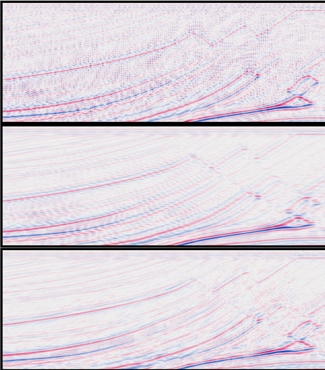
Figure 4 : Comparison of PSDM crude result ( in the top ) without any anti-aliasing correction, PSDM result ( in the middle ) using classical sub-optimal anti-aliasing criteria and finally in the bottom the PSDM result using optimal anti-aliasing criteria.
