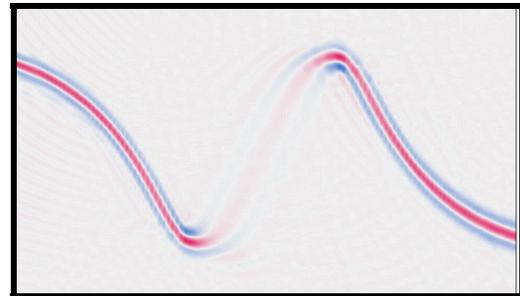
Figure 3 : PSDM result using classical sub-optimal anti-aliasing filtering.
