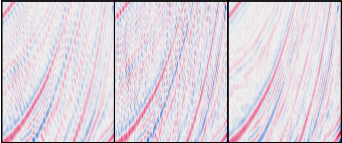
Figure 5 : Close-up of crude PSDM result without anti-aliasing filtering (in the middle) in comparison to PSDM result using standard anti-aliasing criteria (on the left) and to PSDM result using optimal anti-aliasing filtering criteria (on the right).
