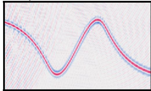
Figure 2 : PSDM result without anti-aliasing protection.
