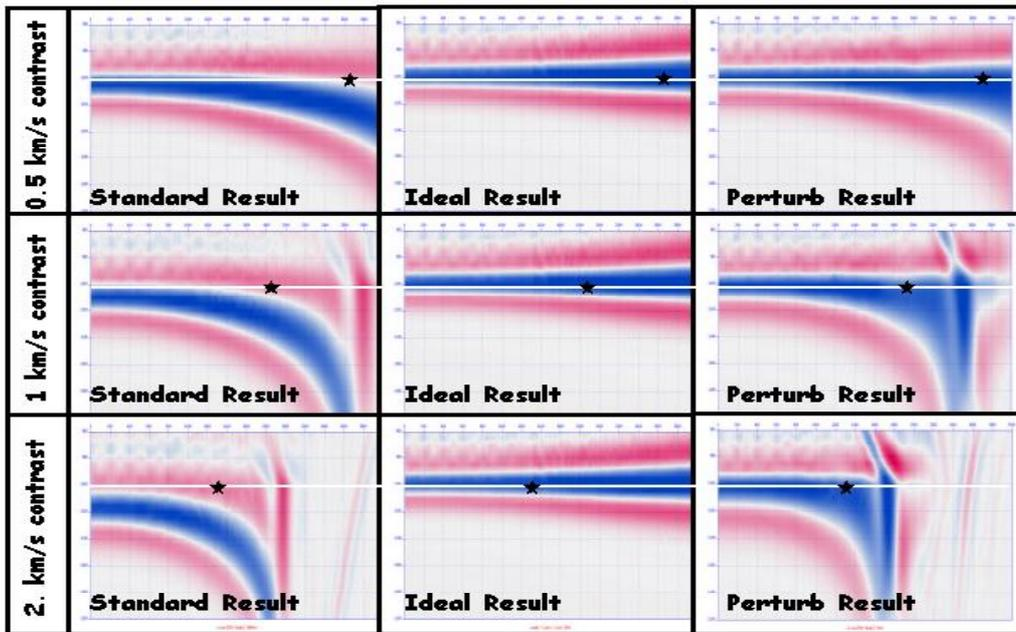
Figure 1: Comparison of Migrated CIG using standard PSDM (left) and perturbation correction (right) for different velocity contrast. In the middle, Ideal migrated CIG using a homogeneous velocity model is reported.
