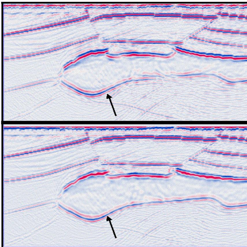
Figure 2: Top :Depth image using the standard (without perturbation correction) PSDM. Bottom : Depth image using traveltimes perturbation scheme.
