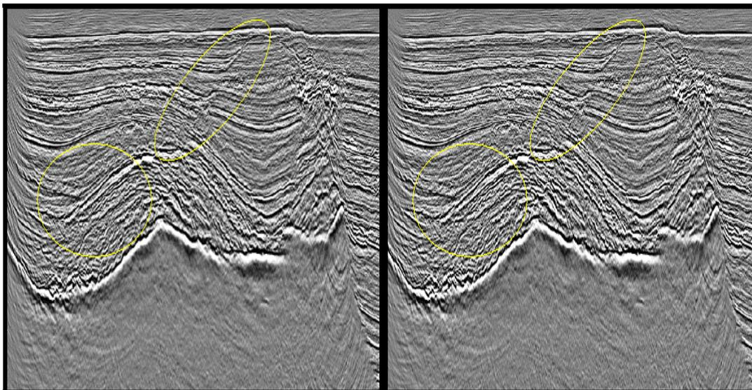
**Figure 4:** Comparison of post migration stack using standard scheme (top) and the new traveltimes perturbation scheme (bottom).
